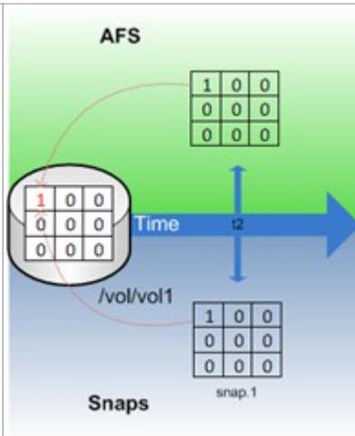
A snapshot named *snap.1* is created. As you can see in the drawing the snap holds pointers to the data blocks the AFS was pointing at the time the snap was taken.
